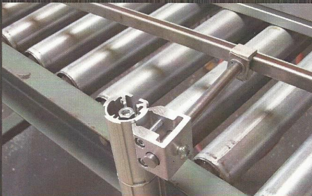
CONVEYOR GUIDE RAIL
