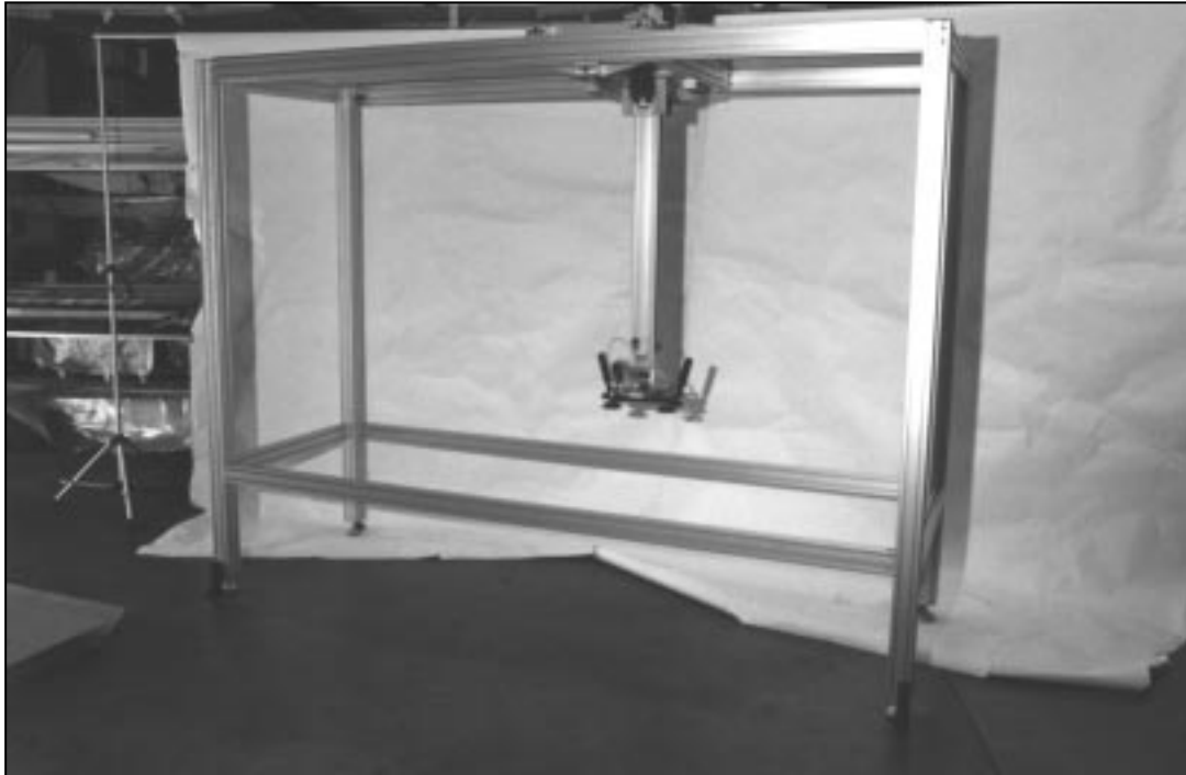
Manual Packing Gantry
